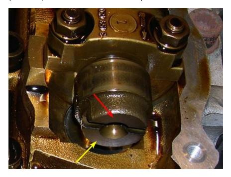
8. If everything is lined up properly and the engine is at Cyl. #1 TDC, you should be able to slide the camshaft locking tool (VW tool #3268) into the grooves. Instead of using the VW tool, I just used two 1/8" thick pieces of Al plate (purchased at Lowe's) to lock each camshaft individually, as shown by the red arrows in the picture below. You can use pretty much any 1/8" thick metal or dense plastic plate for this purpose.
