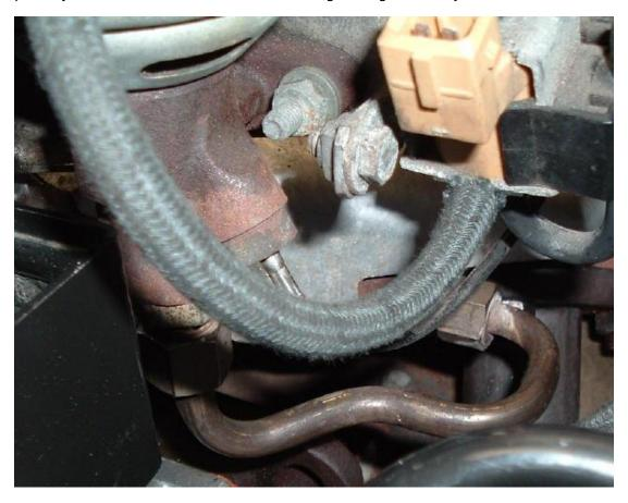
The valve cover can be removed now. If you need to actually remove the EGR valve, first disconnect the vacuum hoses and electrical plugs if not already done. Mark the hoses or make notes to help you reconnect them to the right places later. Then remove the exhaust tube.
