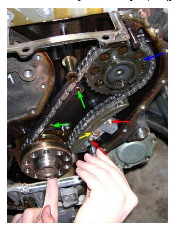
34. Install the new lower timing chain onto the crankshaft sprocket, slide it into the lower guide rail and then over the inner
