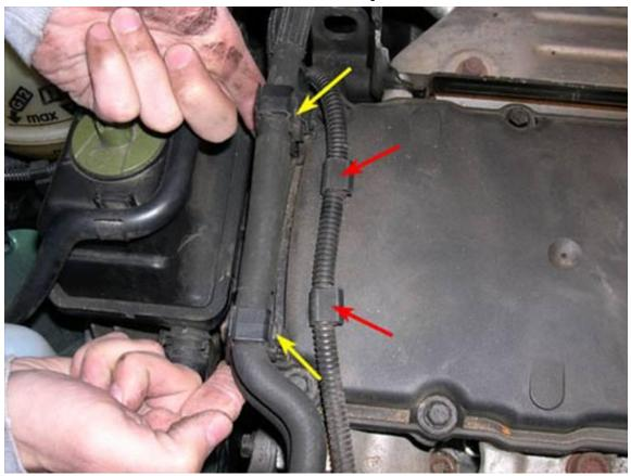
2. Loosen and/or remove the ten (10) 10mm bolts/nuts that secure the valve cover. On a MKIV, there are 8 captured bolts (yellow arrows in picture below) and 2 nuts on posts (red arrows in picture below). I believe that all ten are nuts on posts on other VR6 engines, but I may be wrong. Once the valve cover is unsecured, pull it up and off of the head, being careful not to damage the cover gasket (it will be reused).
