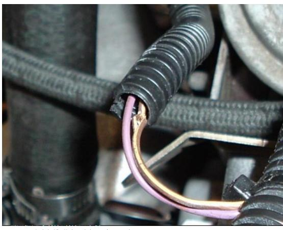
You will notice that I have covered most of my harness with pieces of nylon split loom. The original friction tape wrapping was crumbling into dust and the wiring was in danger. This should be done to prevent having to buy a new engine harness sometime later. Remember that a used harness is going to be old and dry too!
