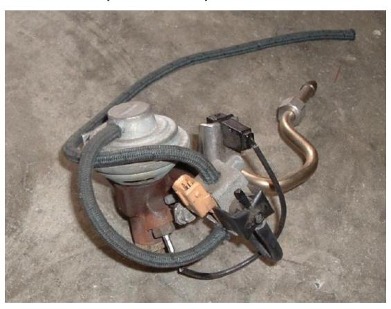
With the EGR system disconnected or out of the way, you can swing the engine harness back up behind the motor if that will get it out of your way. Be very careful handling the wiring. Engine heat makes wires brittle and you get insulation cracks like this one.
