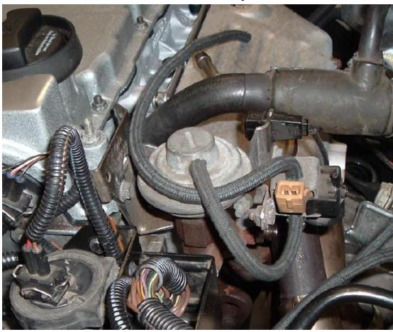
As you can see, you will need to disconnect the engine wiring in the upper area so that the harness can be folded back to the driver's side out of your way.
