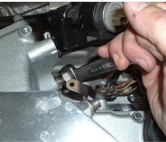
To remove the valve cover, you will have to unbolt the EGR assembly from it. It is attached using two 10mm hex head bolts that go through a wiring harness support as well as the EGR bracket. You can see one of the bolts in the pic, the other is behind the vacuum hose.
