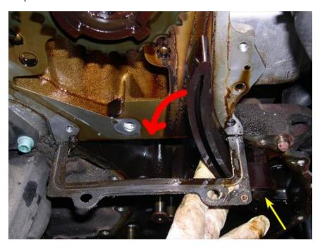
25. To remove the upper tensioner rail, simply slide it off of the pivot pin, as indicated by the yellow arrows in the picture below. You do not need to remove the pivot pin.
