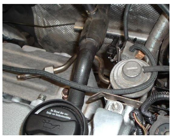
There is very little room so you will have to use the open end of your 10mm wrench to back these two bolts out together a little at a time. There are also two bolts holding the valve to the bracket, but they are no piece of cake either and they would open a gas seal at the intake tube. So stick with the two bolts up front.
