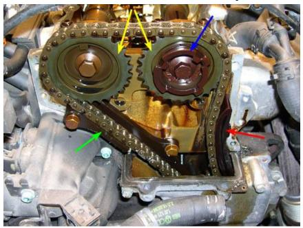
15. The picture below shows a close-up of my original upper guide rail. The yellow shading shows the location of a piece that broke off and was causing the rattling noise heard in the sound clip in the link above. •
