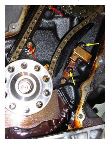
27. Slide the inner intermediate sprocket off of the intermediate shaft (note that the shaft is also keyed so that the sprocket only goes on one way) and then remove the lower timing chain from the crankshaft sprocket. Finally, slide the lower guide rail off its guide pins, which are indicated by the red arrows in the picture above. You do not need to remove the guide pins.
