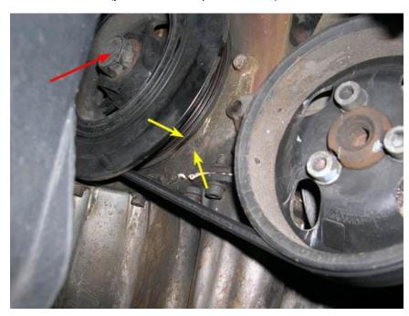
NOTE: When doing gross rotations of the crankshaft, always turn the crankshaft the same direction that it rotates when the engine is running (clockwise in the picture below). It's OK to rotate it the opposite way for small adjustments only.
