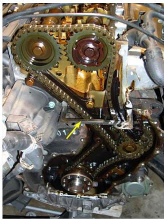
20. Remove the upper guide rail by removing the two (2) 13mm bolts (yellow arrows in picture below) and then sliding the rail up and off of the lower guide post (red arrow in picture below). You do not need to remove the guide pin. (Note that the guide pin resides behind the lower chain cover - I suspect that VW used a guide pin instead of a bolt here so that the guide could be replaced without having to remove the lower cover, and consequently, the tranny, clutch, etc).
