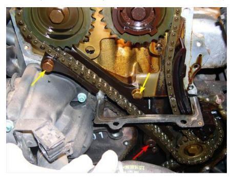
NOTE: If you are only replacing the upper guide rail, perform step 29 and the appropriate portion of step 35 to install the new guide. Once the guide is installed, perform the engine timing check in steps 40 through 43. Finally, perform steps 48, 49 and 51 through 57 to reassemble everything.
