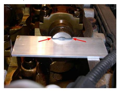
NOTE: Leave the VW or other improvised camshaft locking tool in place in the camshaft grooves until instructed to remove it. This will keep the camshafts from rotating when the upper chain is removed, maintaining the correct valve timing.
