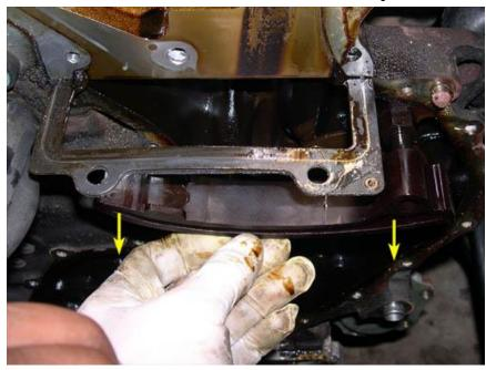
26. Remove the lower tensioner unit by removing the two (2) 5mm hex bolts indicated by the yellow arrows in the picture below (the tensioner will fully extend when removed if you don't hold the rail and body together or secure it with a U-clip like the one that comes with a new tensioner).
