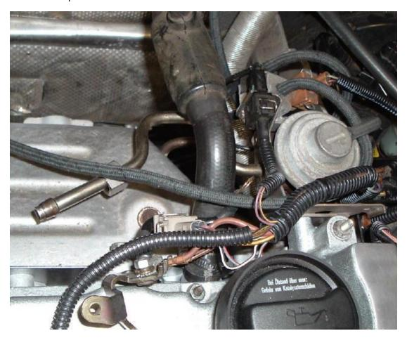
This leaves only the electrical plugs and vacuum lines to connect to the EGR. These can be connected along with the other connections in that area at your convenience. Use zip ties to tie the harness to the support bracket as shown in the first several pictures.
