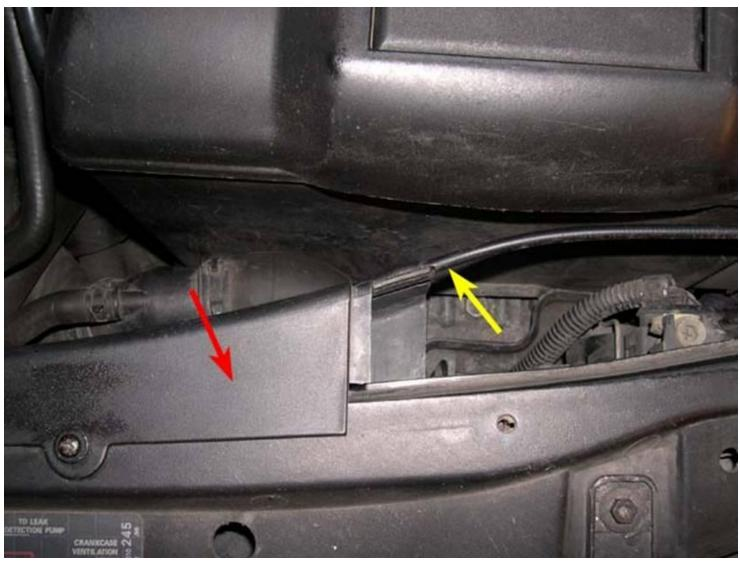
4. Carefully pop the spark plug wires (yellow arrows in picture below) out of their grooves in the small engine cover (red arrow), remove the one (1) T30 screw (green arrow) and remove the engine cover piece (some wiggling may be necessary to get it out from under the wires).
