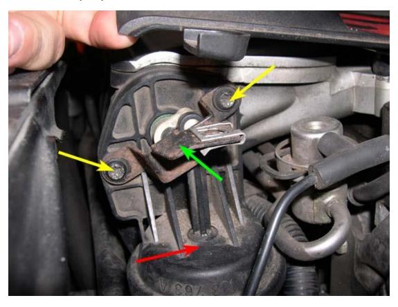
11. The picture below shows a better view of the vacuum drive unit (which also serves as the driver's side end cap) and how
