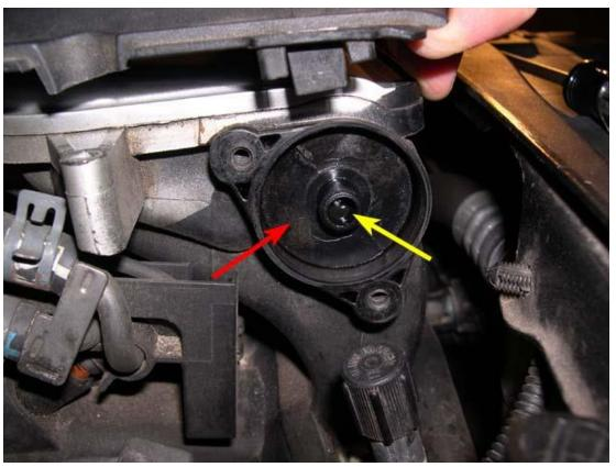
10. The picture below shows the shifter rod's vacuum drive unit (red arrow) on the driver's side of the upper intake manifold. Remove the support bracket (green arrow) for the small engine cover piece (already removed) by removing the two (2) T30 screws marked by the yellow arrows.
