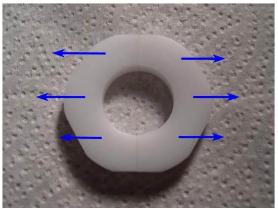
31. The two halves are secured by small pins (red arrows in picture below) and need a light tug to be separated.
