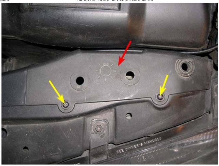
3. Pop the hood release cable (yellow arrow) out of its groove in the trim piece (also part of the stock intake) marked by the red arrow in the picture below.
