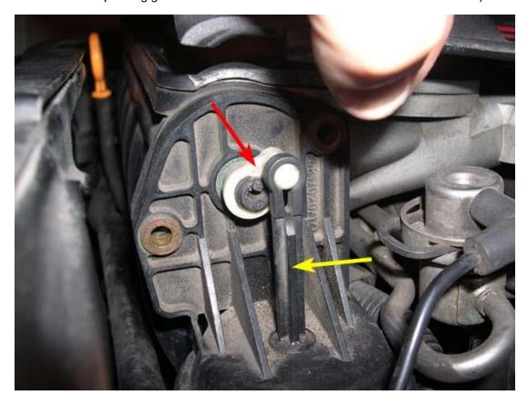
12. The red arrow in the picture below points to the locking tab that secures the white connecting lever to the shifter rod. In order to remove the drive unit from the manifold, the lever needs to be disconnected from the shifter rod. This is accomplished by depressing the locking tab and separating the lever and rod.
