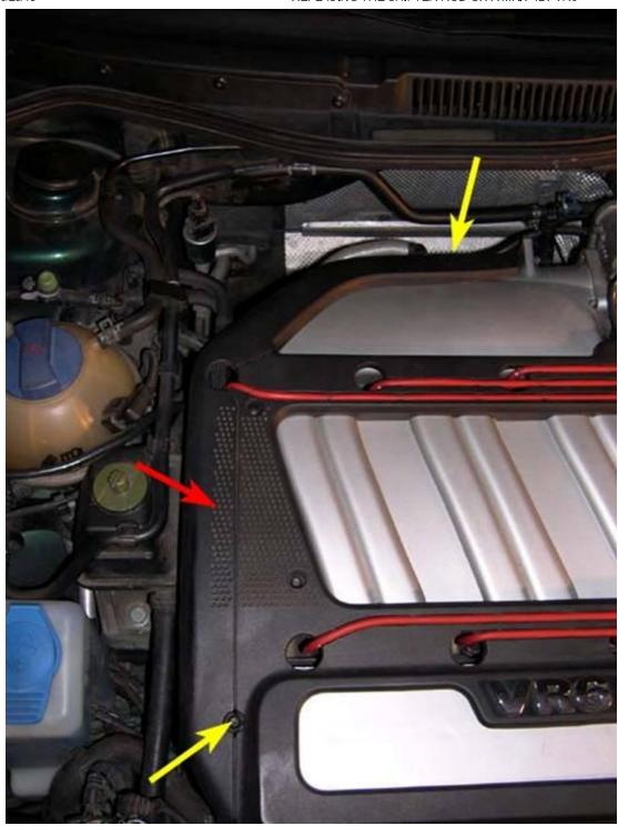
7. Remove the passenger's side end cap for the shifter rod (red arrow in picture below) from the side of the upper intake manifold by removing the two (2) T30 screws (yellow arrows) and then pulling the end cap off. The lower screw may be partially blocked by the A/C service port marked by the green arrow. You can carefully hold this port to the side to access the screw (it will be tough to do most likely), but don't be too rough with it. Just move it enough to get the screw out.
