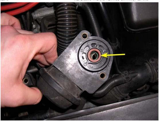
17. Finally, slide the shifter rod out of the driver's side of the intake manifold, as shown below. If the bushings on the rod are worn, it will slide out very easily and it will become very clear why the rod rattles so badly in the 2500-4000 RPM range. If your shifter rod still has a tight fit in the manifold (doubtful), then you might need to lightly tug on the rod to get it out. Be careful not to cut your fingers as some of the edges of the rod can be sharp!
