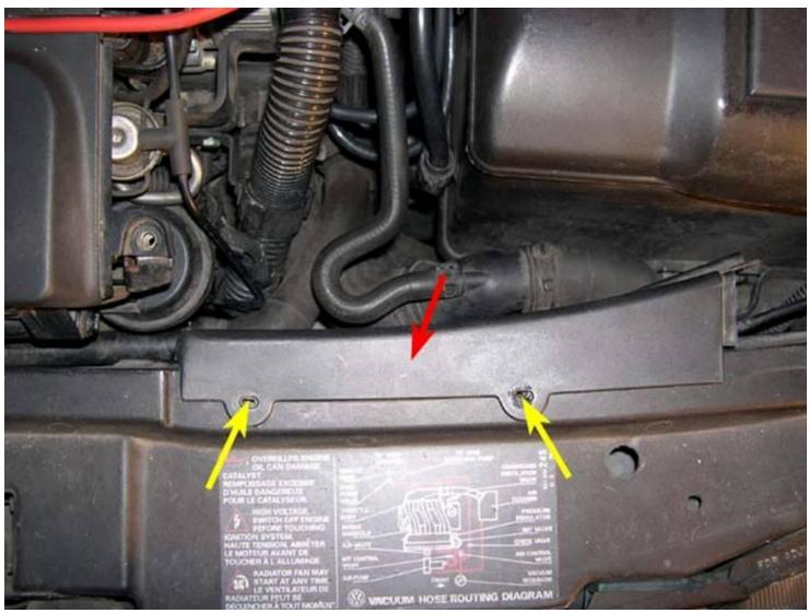
6. Remove the long, thin engine cover piece on the passenger's side of the engine (red arrow in picture below) by removing the two (2) T30 Torx screws (yellow arrows) and carefully pulling up on the trim piece.
