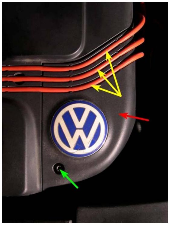
5. Remove the trim piece marked by the red arrow in the picture below by removing the two (2) Phillips screws (yellow arrows) and then sliding the trim piece toward the rear of the car and then up and out. The hood release cable may catch on the inside surface of the trim piece while doing this, so some wiggling may be required.
